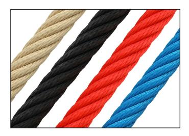
Each of the six outer strands are made of a 2.8 mm galvanized steel wire cable, coated by a 1 mm layer of high-strength polypropylene. The cable is jacketed with a protective layer of high-strength UV resistant polyester fiber for a total single-strand thickness of 5.8 mm.
