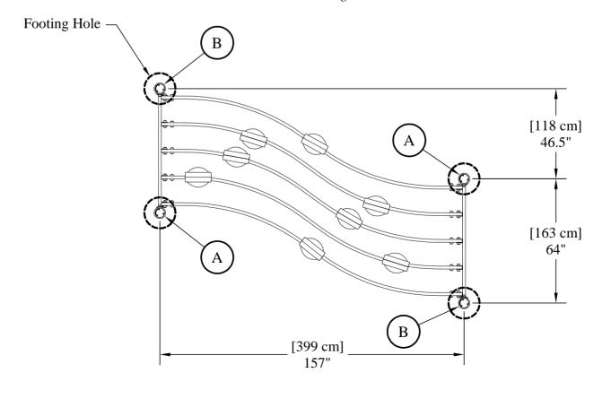
3. **Attach Brackets** (D) to columns (A)(B) using hardware (G)(L)(H)(M) as shown. Do not install Do-Nut Caps (I) until installation is complete and all hardware are tightened.
