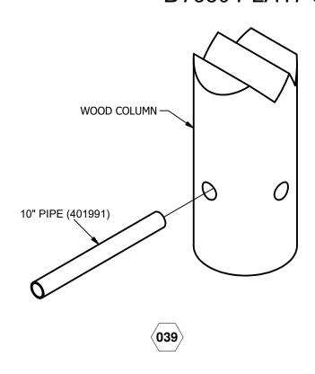
NOTE: REFER TO THE INSTALLATION PROLOG FOR TYPICAL THREADED INSERT AND EAGLE FASTENER INSTALLATION.
