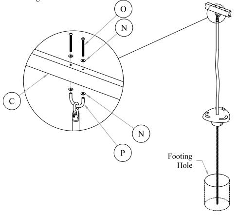
17. **Fill each PlayPod Footing Hole** with concrete while restraining the lower chain.
