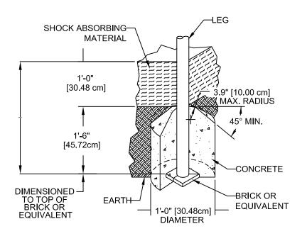
SHOCK ABSORBING PROPERTIES OF SURFACING MATERIALS VARY. IF YOU DETERMINE THAT LESS THAN 1'-0" [30.48cm] OF SURFACING IS REQUIRED, OR IF INSTALLED HEIGHT OF DISH IS TO BE LESS THAN 2'-6" [76.20cm] MAXIMUM, MAKE UP THE DIFFERENCE IN ELEVATION WITH EARTH, BEFORE APPLYING SURFACING.
