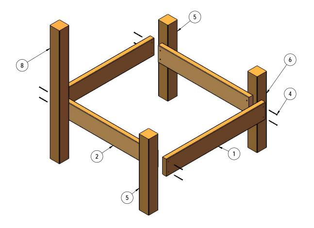
Attach the  $2" \times 6" \times 36"$  Cedar Recycled Planks to the ends of the  $2" \times 6" \times 33"$  Cedar Recycled Planks using the specified hardware.
