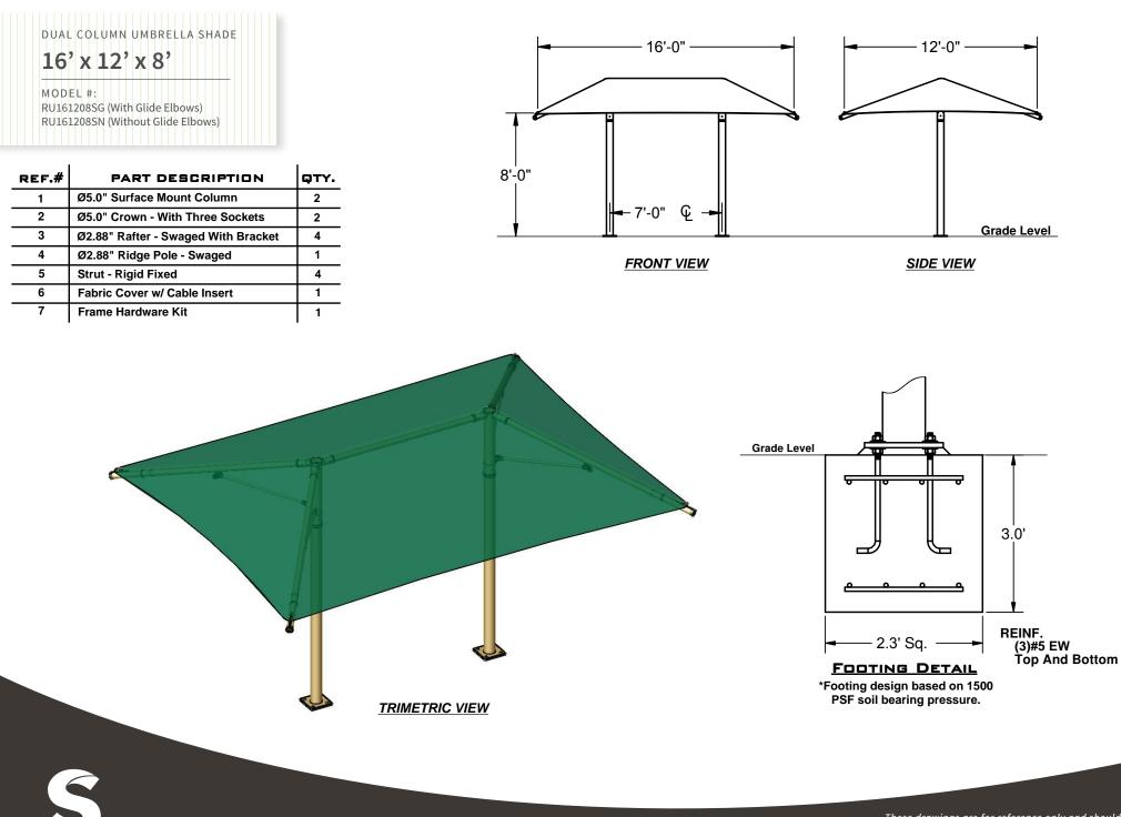
These drawings are for reference only and should not be used as construction details. Materials, fasteners, and foundations are subject to change if professionally sealed engineering drawings are required. Designed for 93 MPH Basic Wind Speed.
