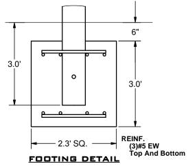
\*Footing design based on 1500 PSF soil bearing pressure.
