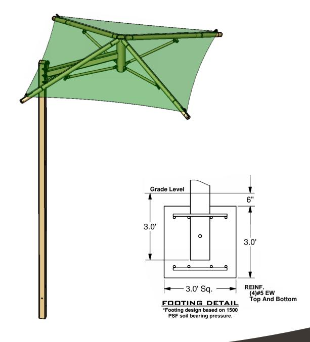
These drawings are for reference only and should not be used as construction details. Materials, fasteners, and foundations are subject to change if professionally sealed engineering drawings are required. Designed for 93 MPH Basic Wind Speed.
