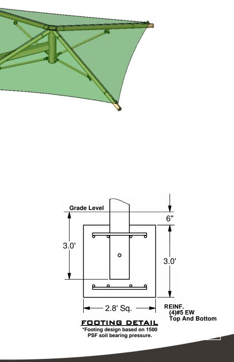
These drawings are for reference only and should not be used as construction details. Materials, fasteners, and foundations are subject to change if professionally sealed engineering drawings are required. Designed for 93 MPH Basic Wind Speed.
